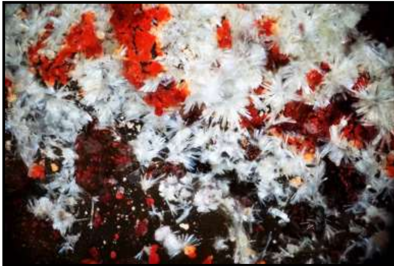
Figure 194. Closeup of exceptional coverage of acicular MCDUK-30 crystal groups. FOV = 0.4 mm.
