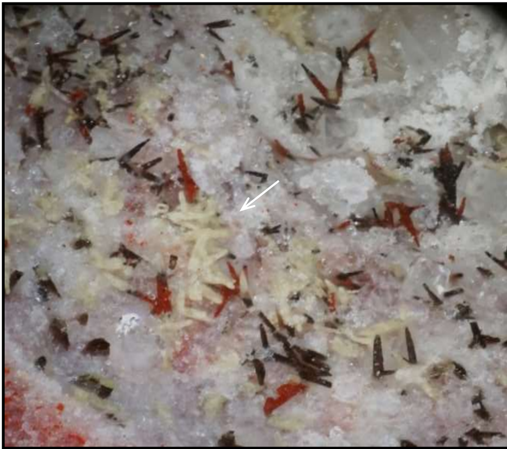
Figure 169. Quartz surface showing prisms of MCDUK-3 with red corderoite coatings. Some have turned black. Note the off-white prisms of MCDUK-3 at arrow. FOV = 1 mm.
