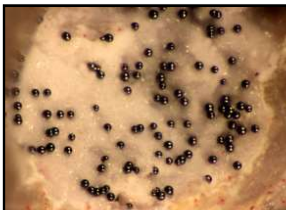
Figure 225. Bright, black spheres of hematite on silica. FOV = 1 mm.
