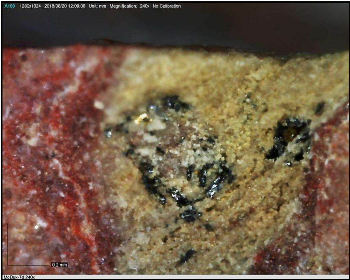
Figure 177. Group of prismatic MCDUK-7 crystals in depression.
