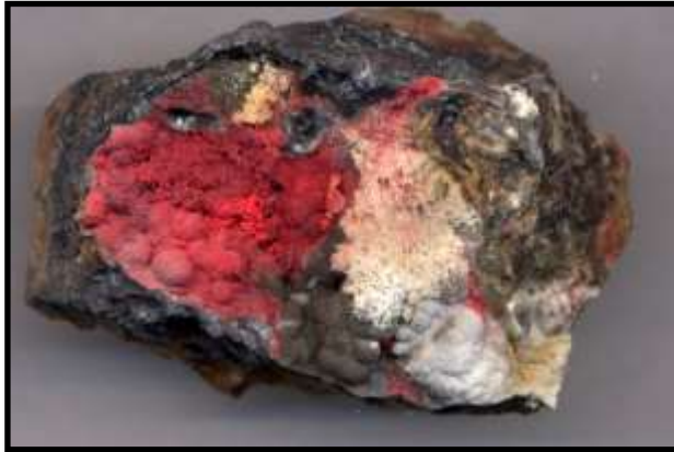
Figure 63. Coating of cinnabar on silica rods with orbicular stibnite underneath. FOV = 60 mm.
