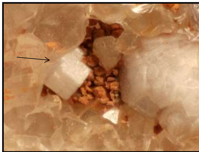
Figure 235. White microcline crystal in cavity of quartz. FOV = 3 mm.
