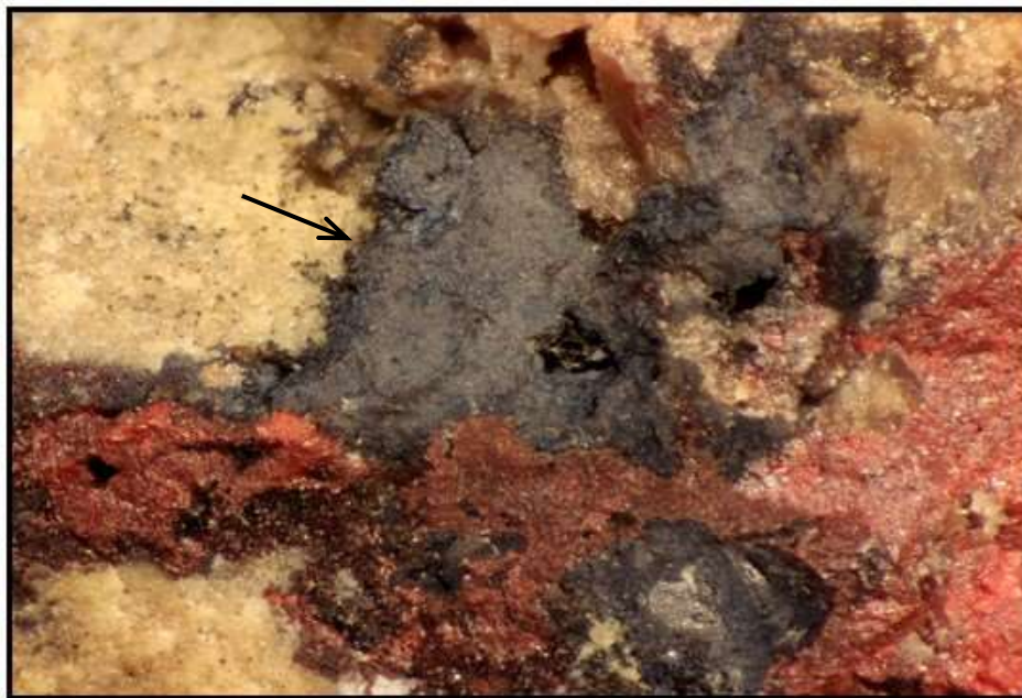
Figure 198. Fine gray replacement product of cinnabar containing minute crystals of corderoite, kenhsuite and \beta -Hg 3 S 2 Cl 2 . FOV = 2 mm.
