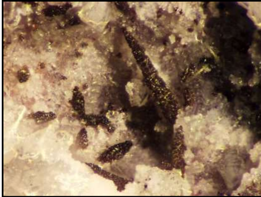
Figure 162. Group of dark brown MCDUK-3 prisms on quartz covered with minute corderoite crystals. FOV = 1 mm.
