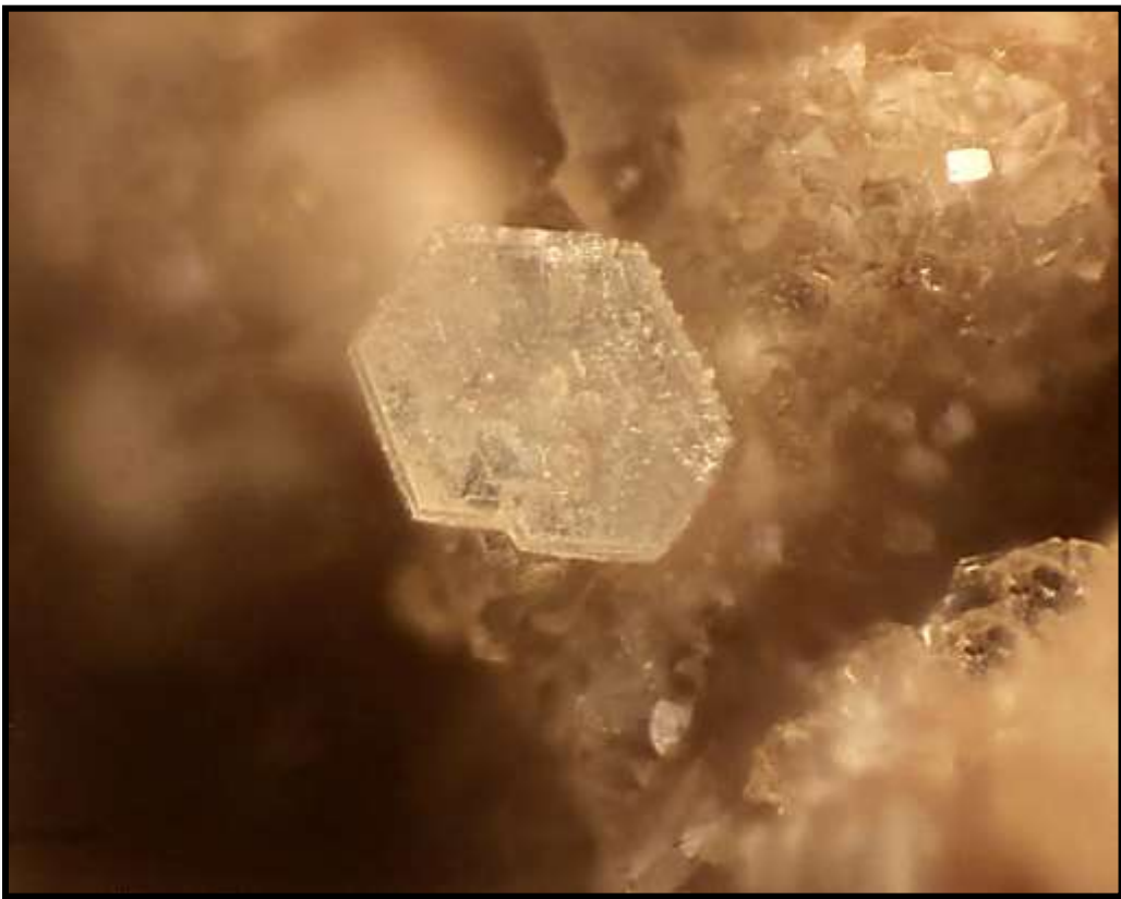
Figure 218. Single hexagonal crystal of fluorapatite. FOV = 1 mm.
