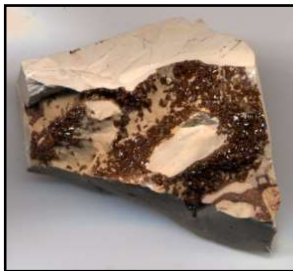
Figure 226 (left) & 227 (right). Coating of dark brown jarosite crystals on altered rock. FOV = 40 mm.
