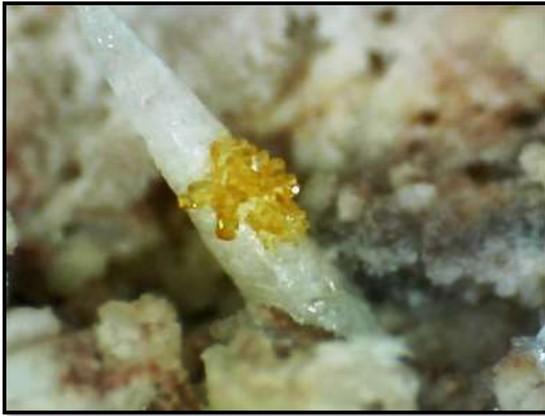
Figure 110. Group of prismatic kleinite crystals on a calcite crystal. FOV = 2 mm.
