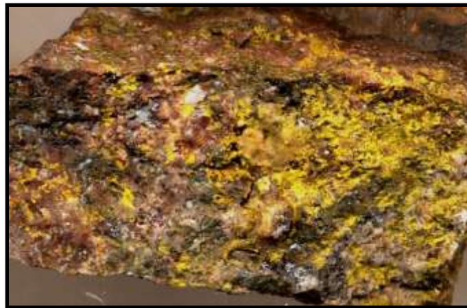
Figure 94. Surface coating of yellow eglestonite. FOV = 20 mm.
