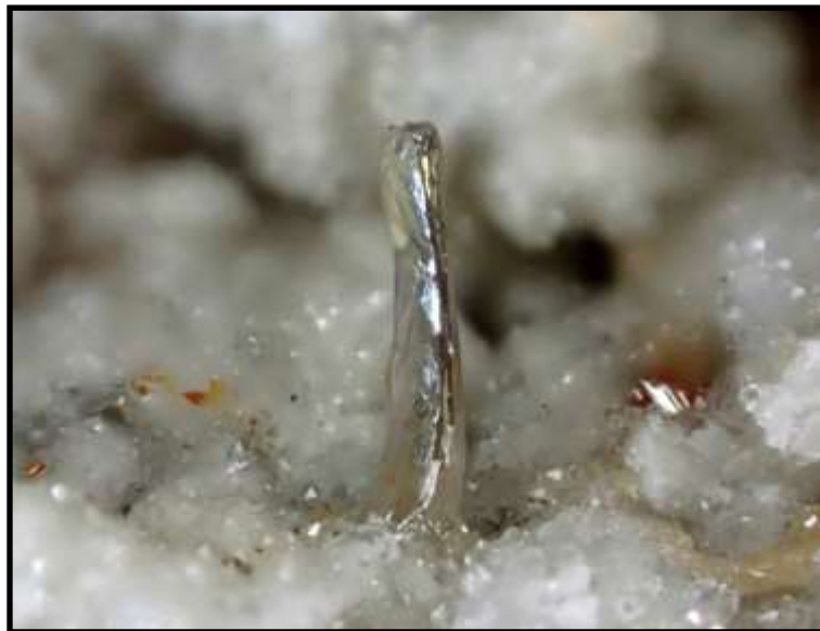
Figure 60. Elongated calomel crystal showing a smooth surface on quartz. FOV = 1 mm.
