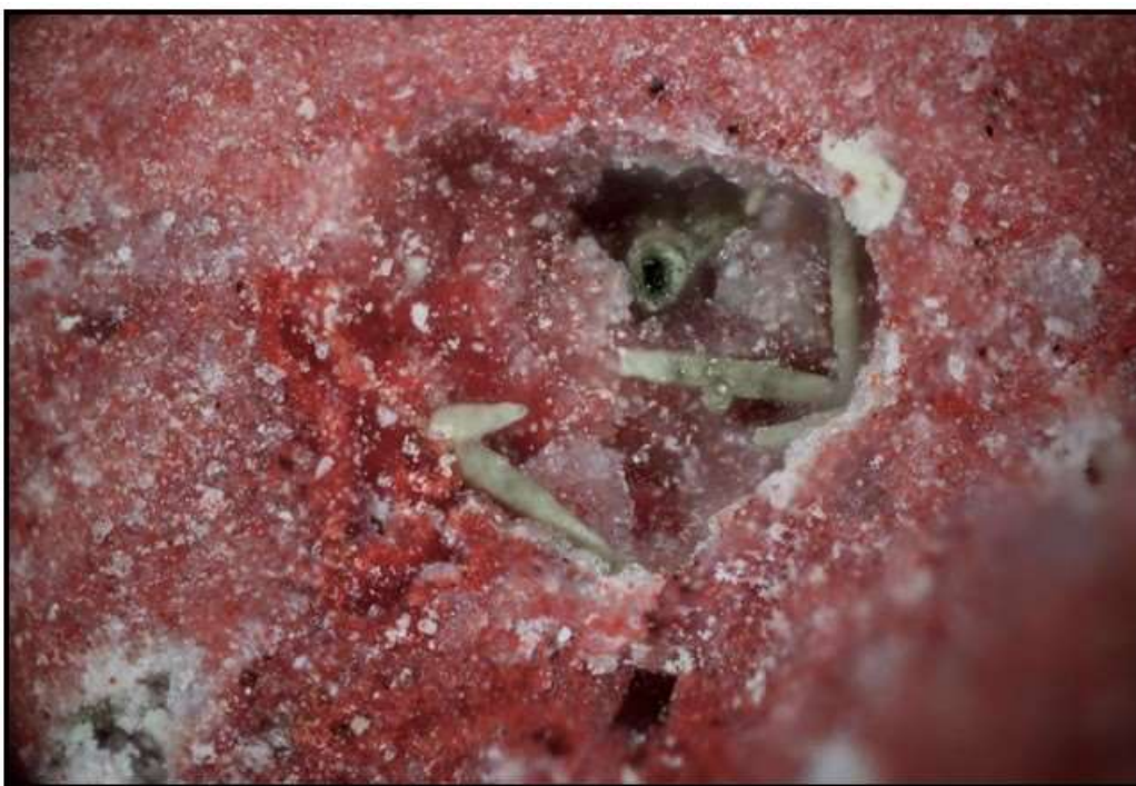
Figure 172. Several MCDUK-3 prisms, one showing dark brown core. FOV = 2 mm.
