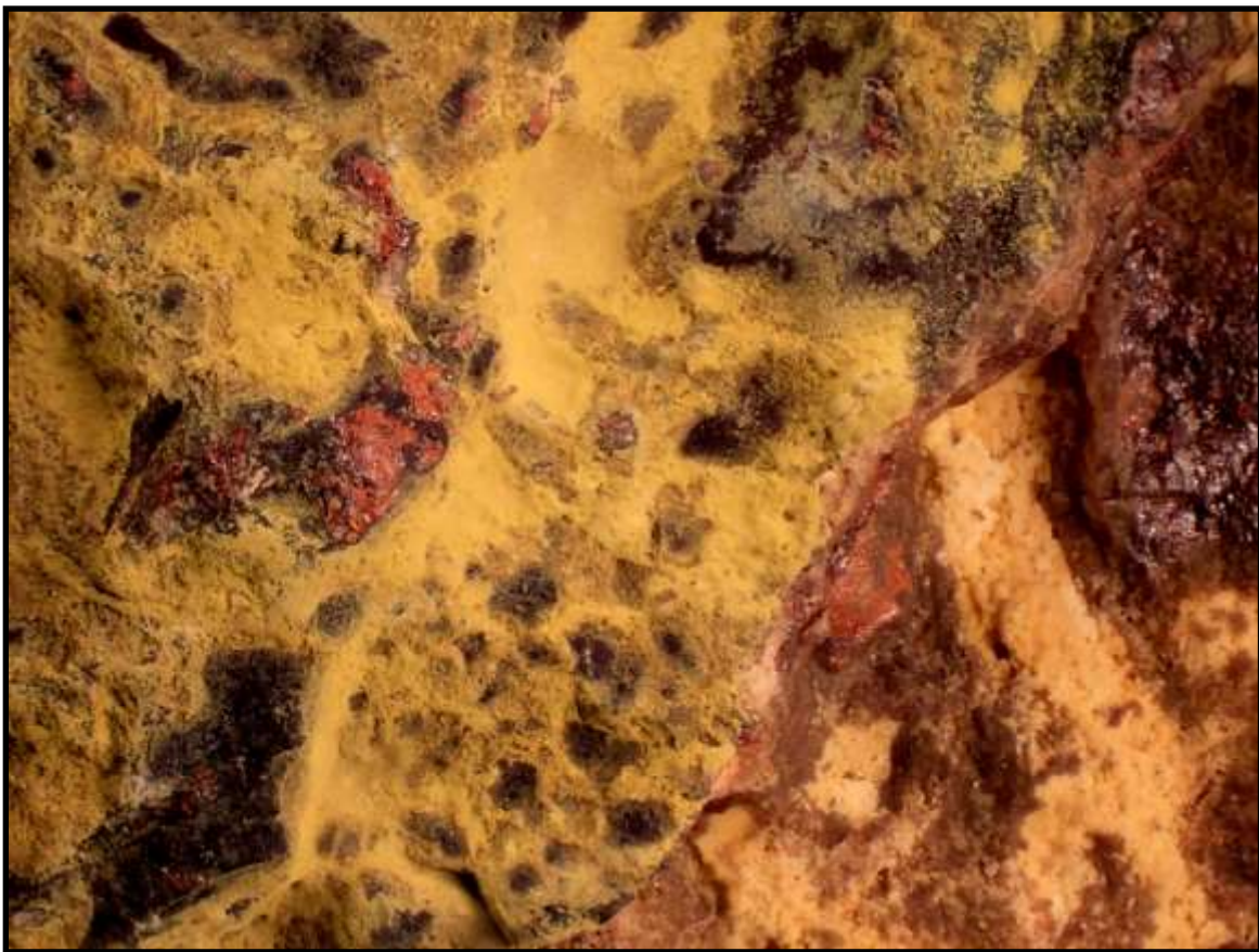
Figure 122. Fine coating of yellow schuetteite on cinnabar. FOV = 3 mm.
