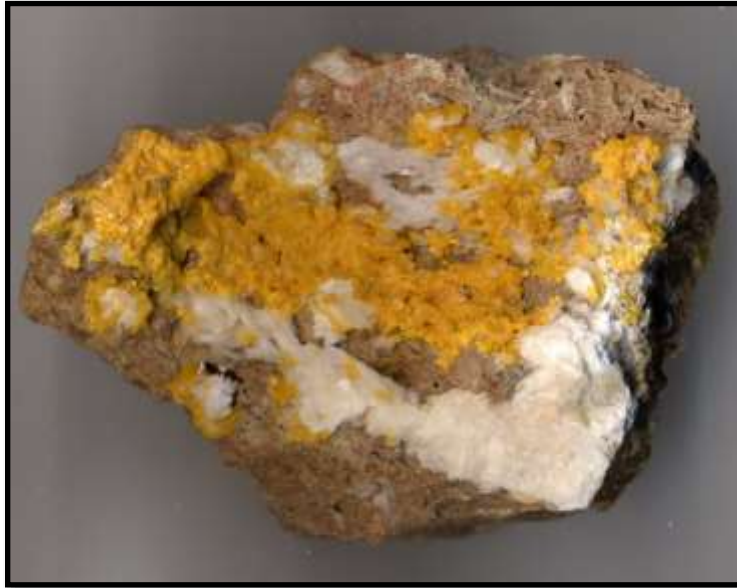
Figure 100. Surface covering of yellow-orange kleinite crystals on rhyolite. FOV = 40 mm.
