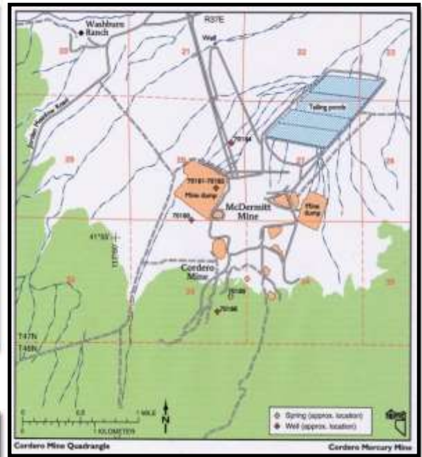
Figure 10. Map showing the proximity of the Cordero and McDermitt mines with dumps and tailing ponds. (after Rytuba and Glanzman 1979).
