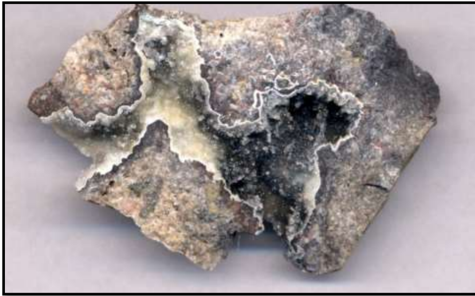
Figure 246. Cavity in silica rock containing thin stibnite crystals. FOV = 60 mm.
