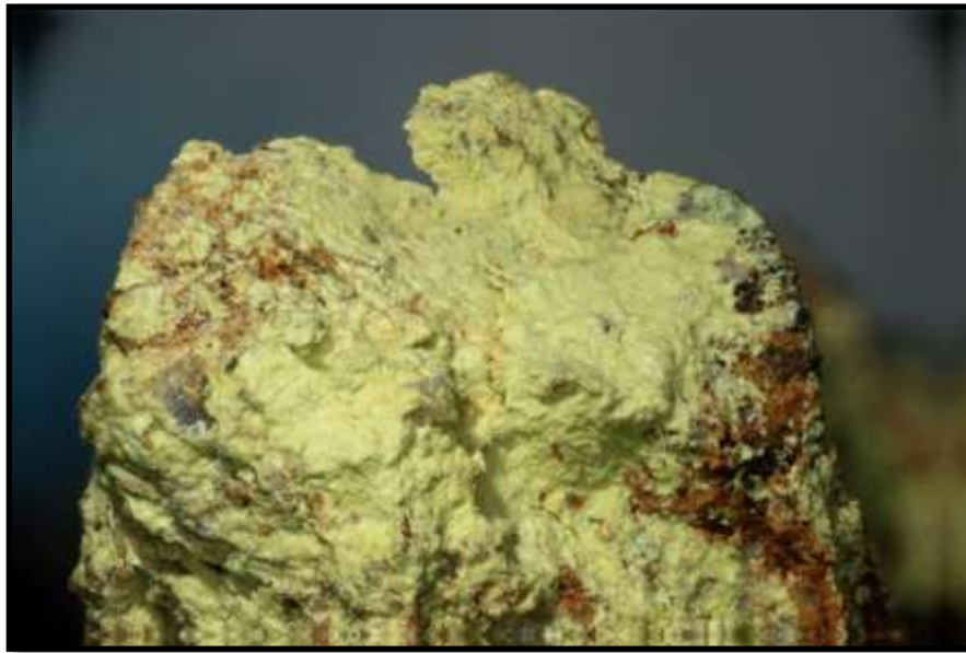
Figure 254. Light green mass of tripuhyite. Photo courtesy of R. Thomssen, FOV = 2 mm.
