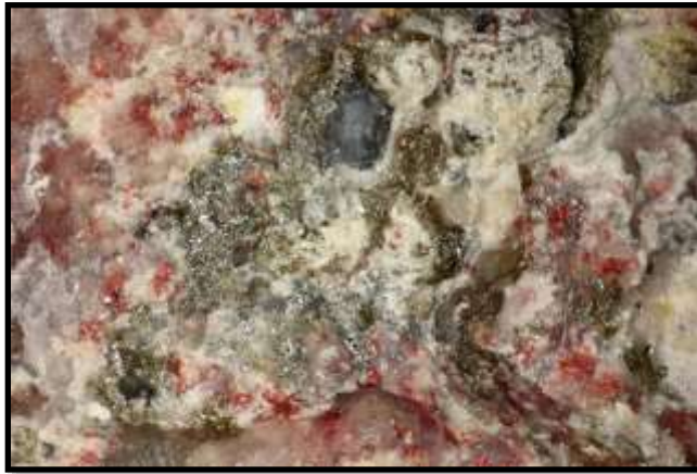
Figure 112. Coverage of mercury with cinnabar. FOV = 3 mm.
