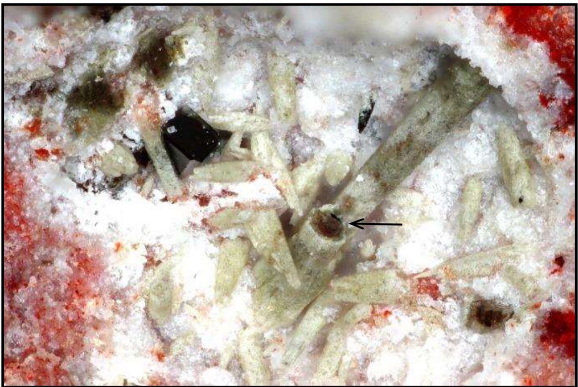
Figure 85. View of single corderoite crystal and several MCDUK-3 prisms. Note the brown core of the prism at the arrow and the hexagonal outline. FOV = 2 mm.
