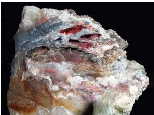
Figure 51. Portion of rock from the productive outcrop. Note the thick massive stibnite vein to the left. In places, this vein has pockets lined with iron-stained drusy quartz and clumps of acicular crystals of light-yellow stibiconite. To the right, the massive stibnite vein gives way to large iron-stained voids that are lined with quartz, chalcedony, and fine-grain cinnabar coating the quartz. The specimen is upside down relative to its in-situ position. The silica lining the large pocket fluoresces a bright green color under ultraviolet light. Horizontal FOV is 29-cm.
