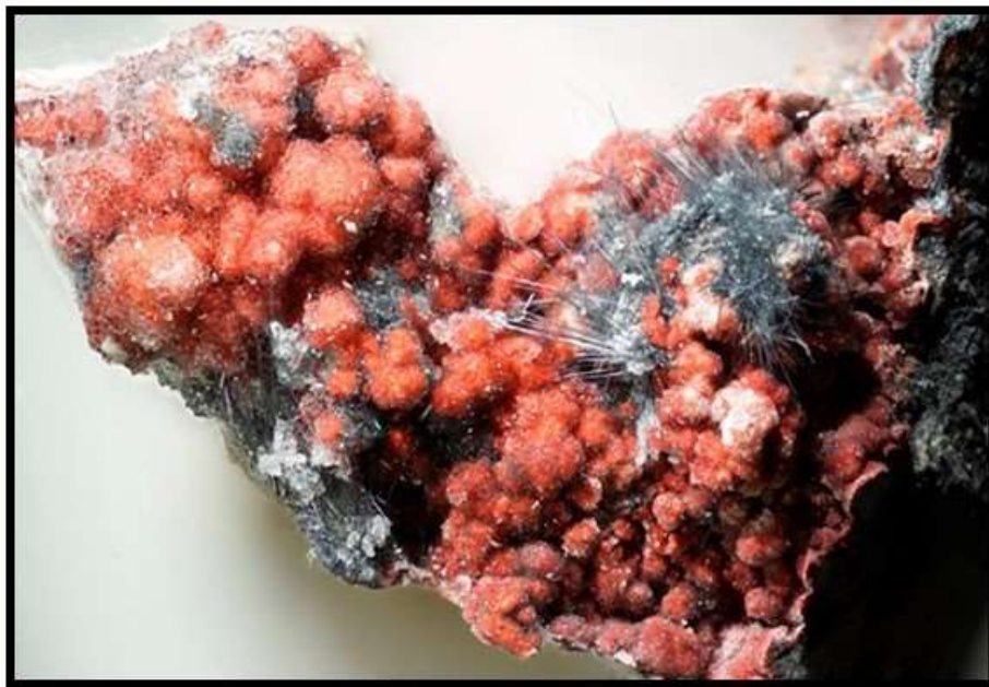
Figure 52. Divergent stibnite needles on silicified tuff and surrounded by orbicular growths of drusy quartz covering cinnabar. Small water-clear double-terminated quartz crystals with valentinite associate with the areas of stibnite, but not the drusy quartz over cinnabar. To the right, out of view, is a dissolution void in a section of massive crystalline stibnite vein. Horizontal FOV is 19 mm.
