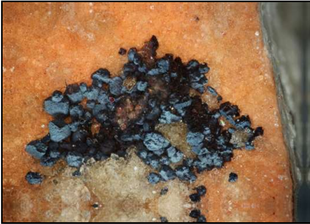
Figure 76. A group of prior cinnabar crystals replaced by corderoite on a quartz base. FOV = 1 mm. The crystals are coated (or replaced) with a dark gray/metallic phase have been identified as cinnabar. The core of these crystals are hollow with a highly reflective silvery phase, which was identified as corderoite. The crystals range in size from 0.5 to less than 0.1 mm. Some crystals show a pyramidal termination, while others show no crystal forms.
