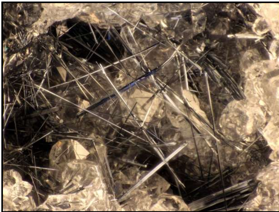
Figure 250. Quartz cavity hosting delicate stibnite crystals. FOV = 6 mm.
