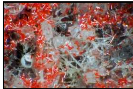
Figure 68. Coverage of silica rods coated with cinnabar. FOV = 2 mm.
