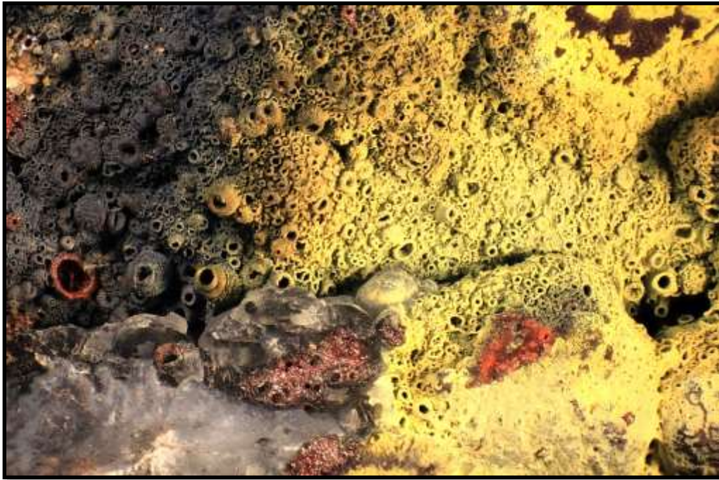
Figure 123. Fine coating of yellow schuetteite on a silica hollow tube matrix. FOV = 6 mm.
