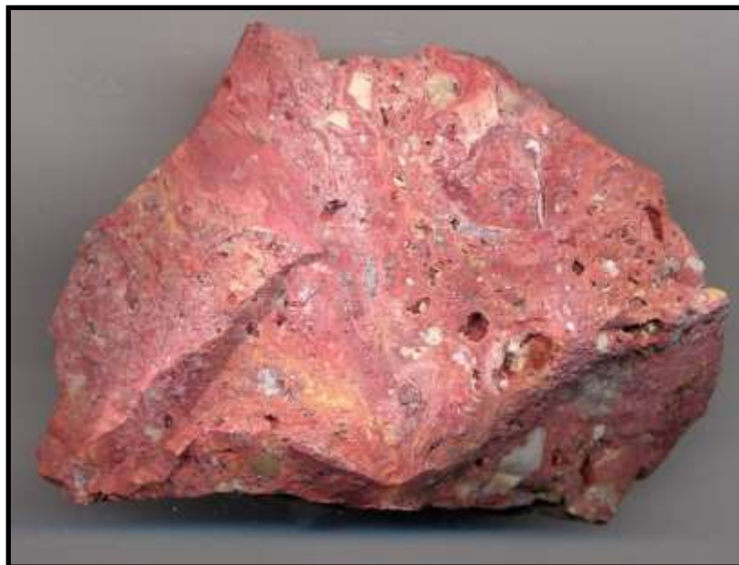
Figure 69. Typical example of freshly broken massive corderoite-bearing rock with high silica content and conchoidal fracture. FOV = 70 mm.
