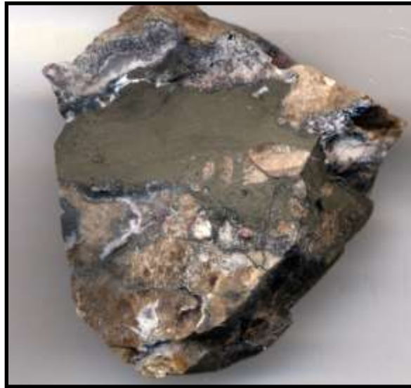
Figure 237. Vein of fine-grained pyrite with stibnite. FOV = 50 mm.
